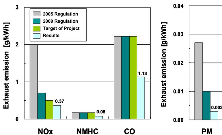
Fig. 9 Emission Test Results (JE-05 Emission Test Mode)
