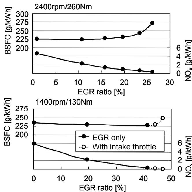
Fig. 6 Effect of EGR on BSFC and NOx
