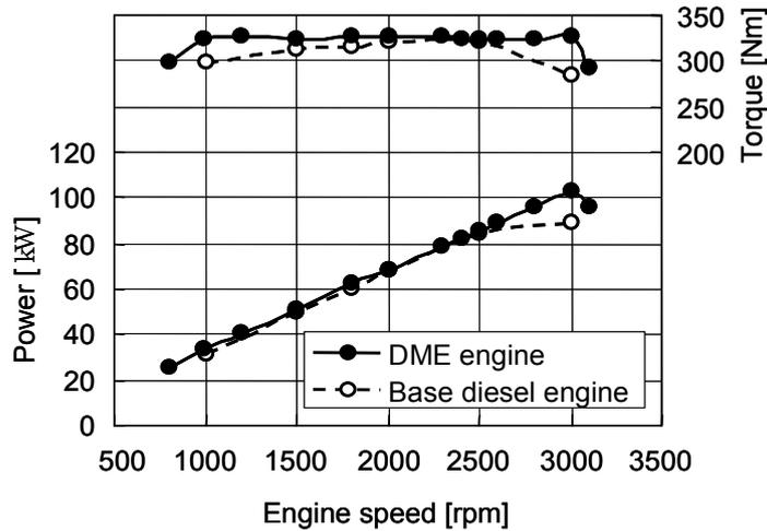
Fig. 5 Engine Output Curve
