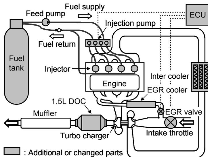
Fig. 2 Outline of DME Engine and Exhaust System
