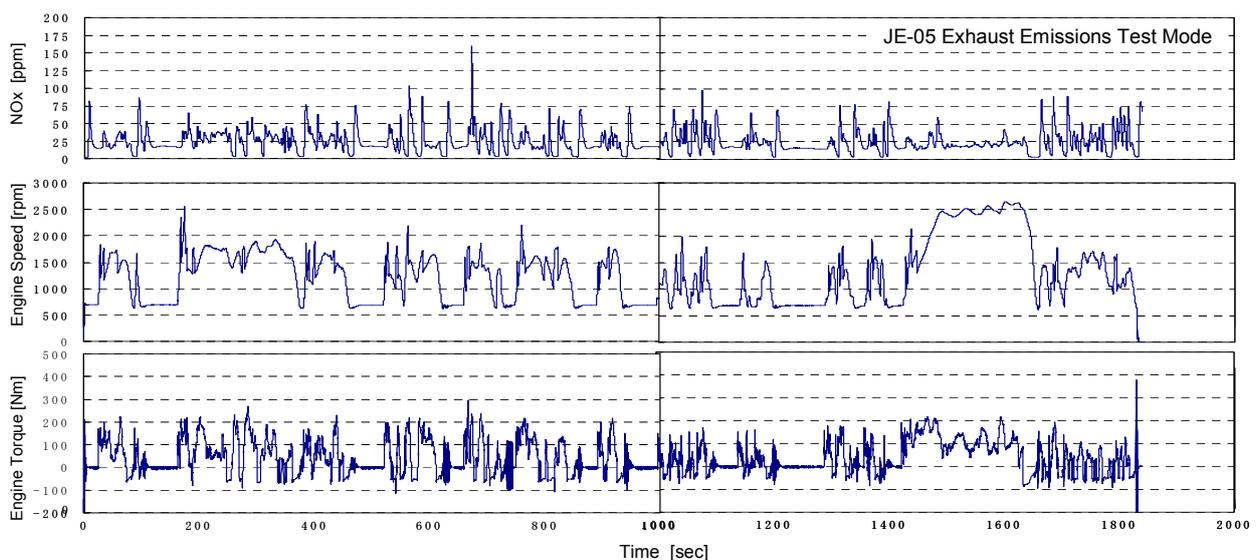
Fig. 8 NO<sub>x</sub> Emission Behavior during JE-05 Emission Test Mode
