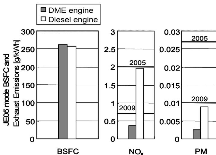
Fig. 10 Comparison of BSFC, NOx and PM (JE-05 Mode)
