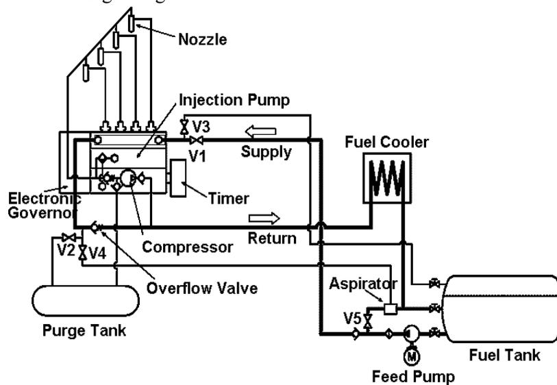
Fig. 3 Configuration of Jerk Type DME Injection System
