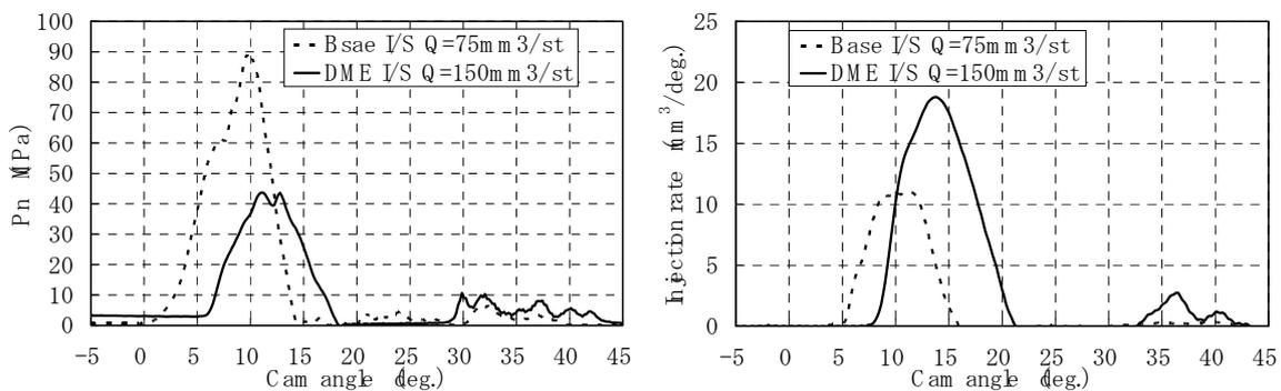
Fig. 4 Comparison of Injection Characteristics
